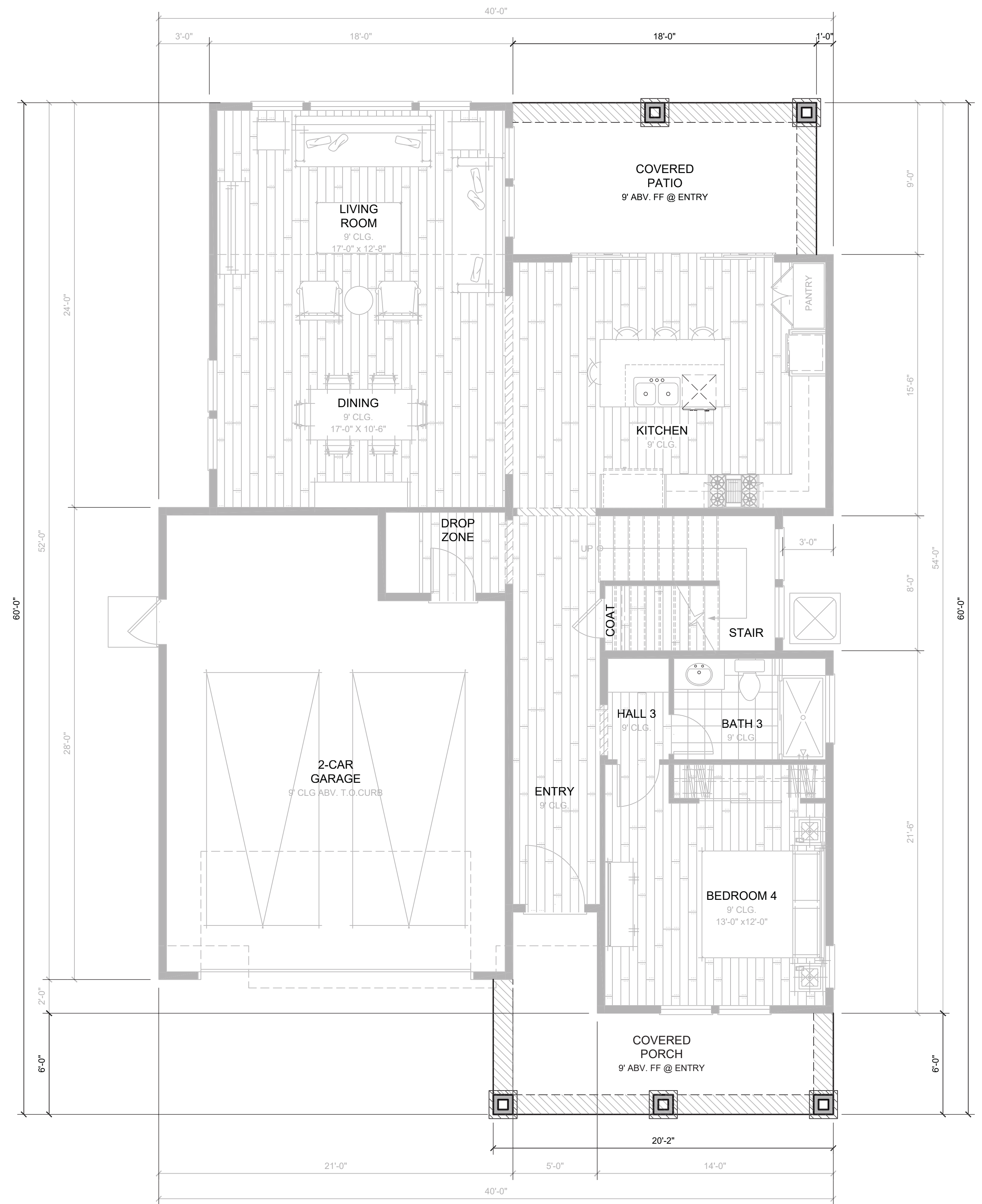
PLAN 1 FIRST FLOOR PLAN, ELEVATION B, CRAFTSMAN SCALE: 1/4" = 1'-0"
